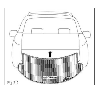
(b) Grasp the tray by the rear and fold in the sides sufficiently to slide it into the rear compartment. After installing the tray, ensure all of the edges are pushed down against the floor (Fig 2-2).
